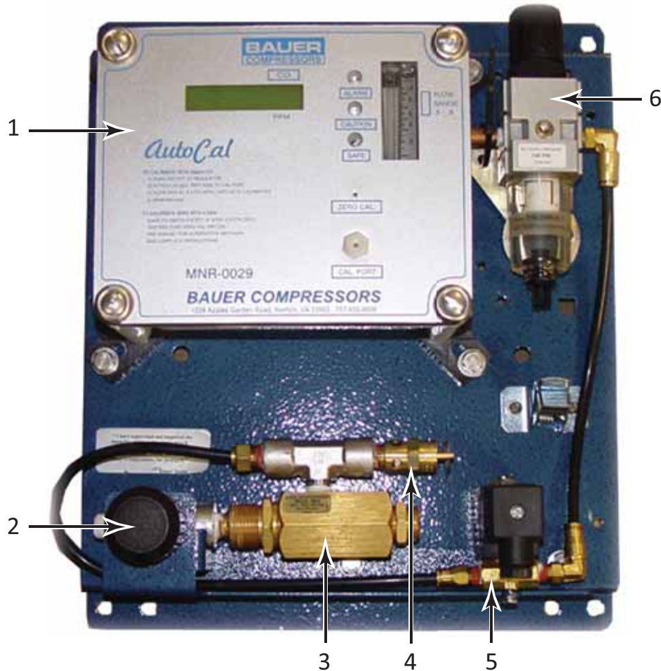
Figure 9-7 Carbon Monoxide Monitor Assembly - TCom Trailer
