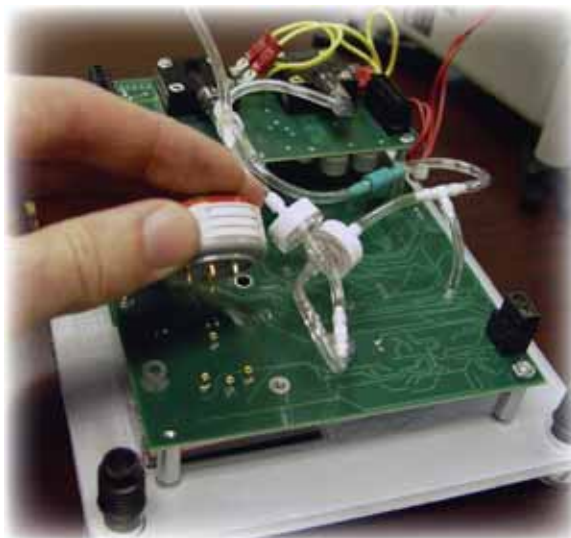
Figure 9-5 Carbon Monoxide Sensor Cell Removal
